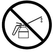
Do not use lubricating oil on the movable parts of the Coin Validator.
