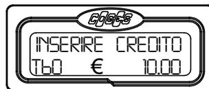
In this last display on the left is shown the time expressed in seconds (ex. T60) which is reduced as the service is distributed.
